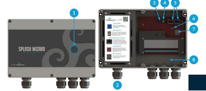
**1. Control Button:** This button, with its distinctive blue ring, acts as the user's main point of control. Pressing will cycle the selected show, and holding will turn the controller on/off.
