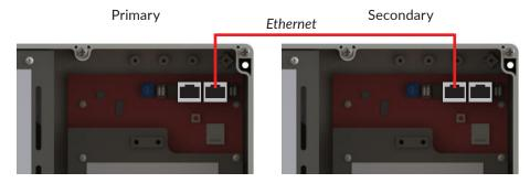
Set the dip switch for the primary and secondary controller, and then connect the output ethernet port of the primary controller to the input ethernet port of the secondary controller.
